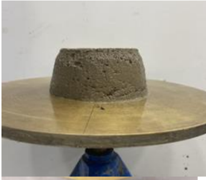
After lifting the cone
