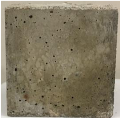
Full cube casting on one pouring
