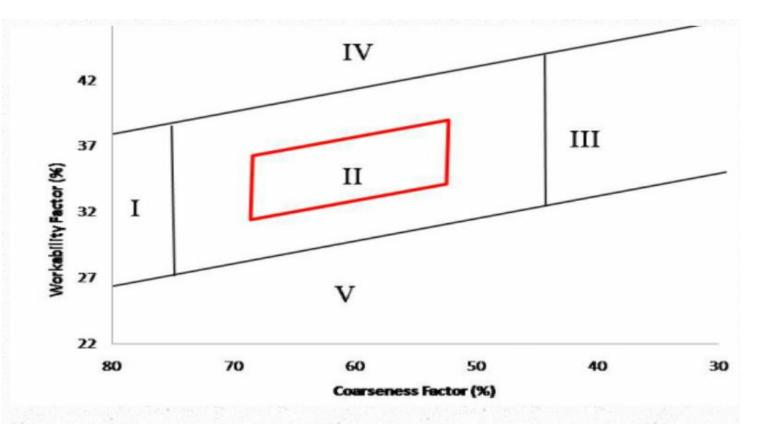
Coarseness Factor (CF) = (Q/R)\*100Workability Factor (WF) = W + (2.5(C-564)/94)
