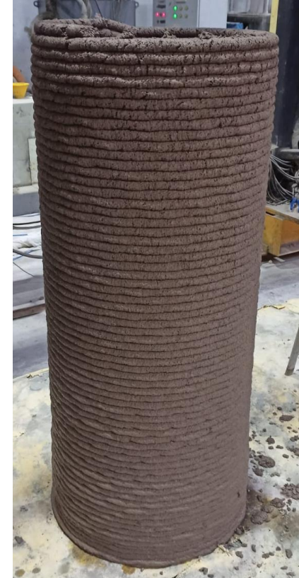
1 m high cylinder – aggregate/binder = 3
