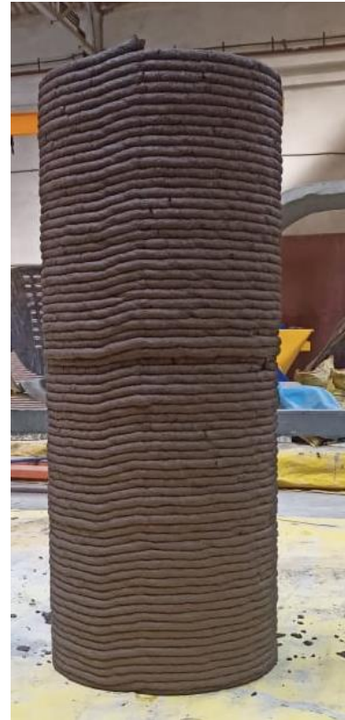
1 m high cylinder – aggregate/binder = 2.33
