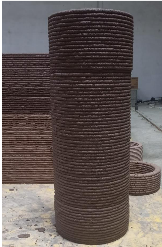
1.1 m high cylinder – aggregate/binder = 1.5
