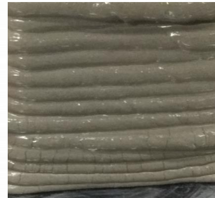
Squeezing of bottom layers
