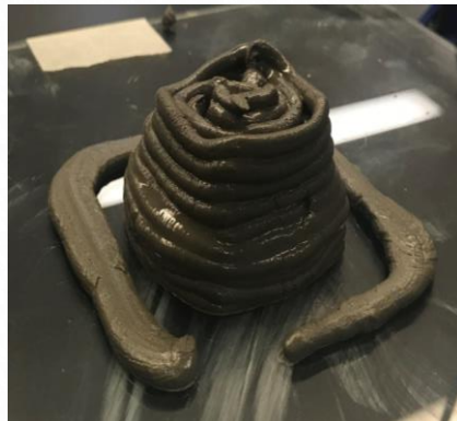
Slumping of printed mixture
