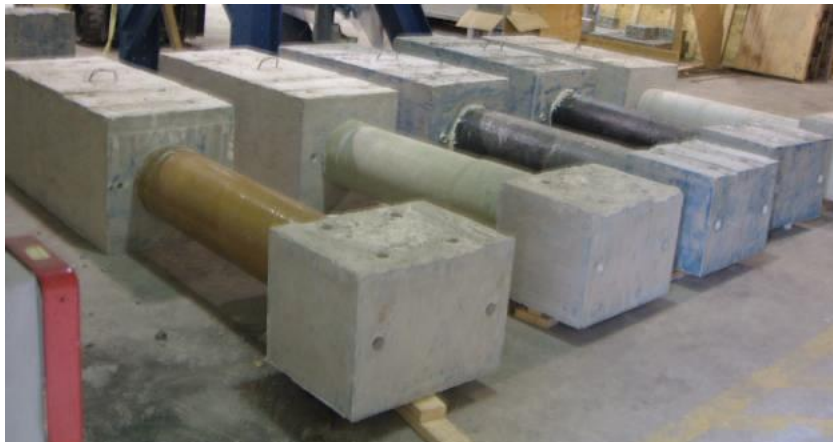
FIU Large-Scale Bridge Pier Specimens with Various FRP Shells (Shi 2009)
