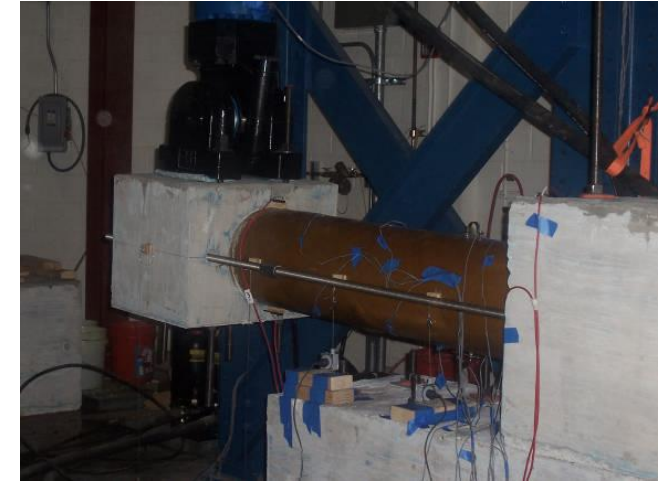
FIU Large-Scale Bridge Pier Cyclic Tests (Shi 2009)
