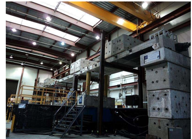
UNR Four-Span Large-Scale Bridge Shake Table Tests (Kavianipour 2013)
