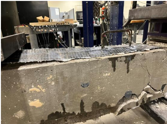
Figure: CFRP sheet debonding and rupture
