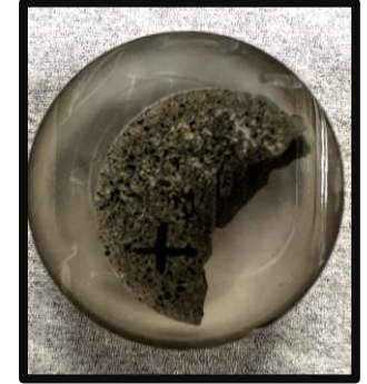
Fig.2. Lunar Concrete (Geopolymer)
