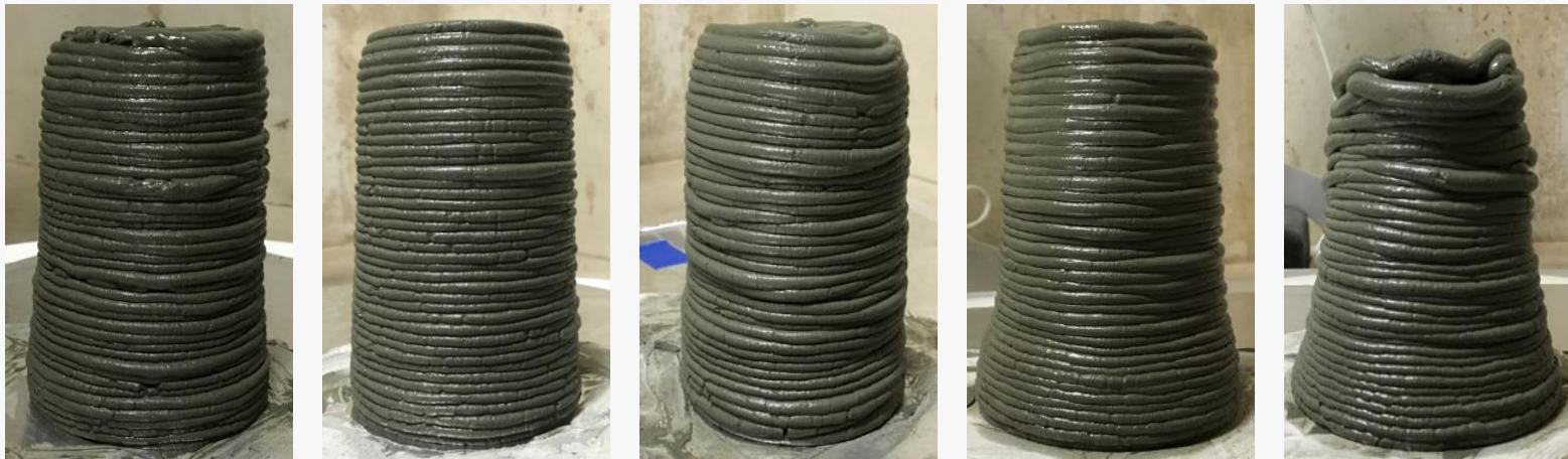
3D printed concrete with different mix proportions
