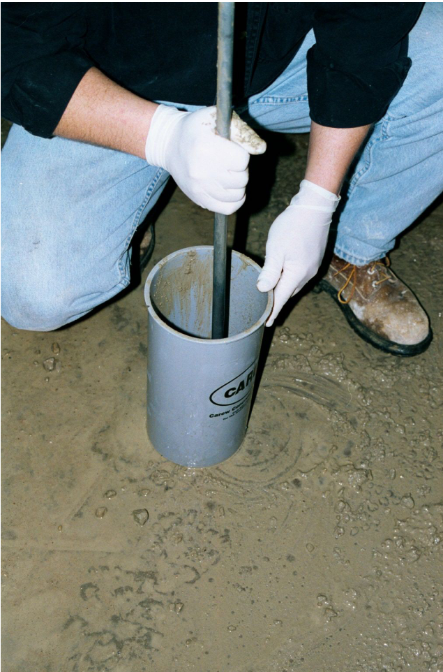
Fig. 0.4—Rodding is performed using a tamping rod, the length and diameter of the rod may vary based on the size of the sample being consolidated (photo courtesy of PCA)
